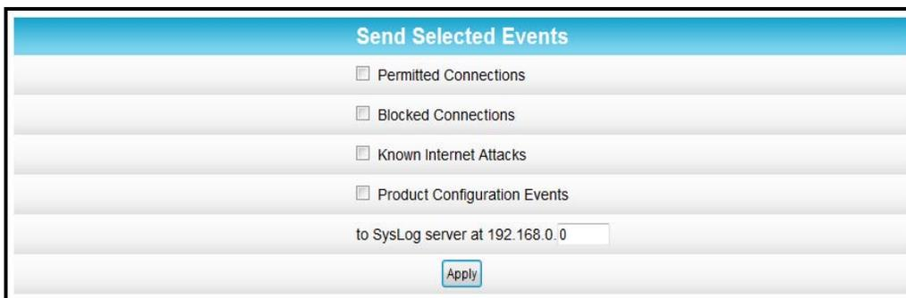
**Figure 31 – Firewall Remote Log Screen**
