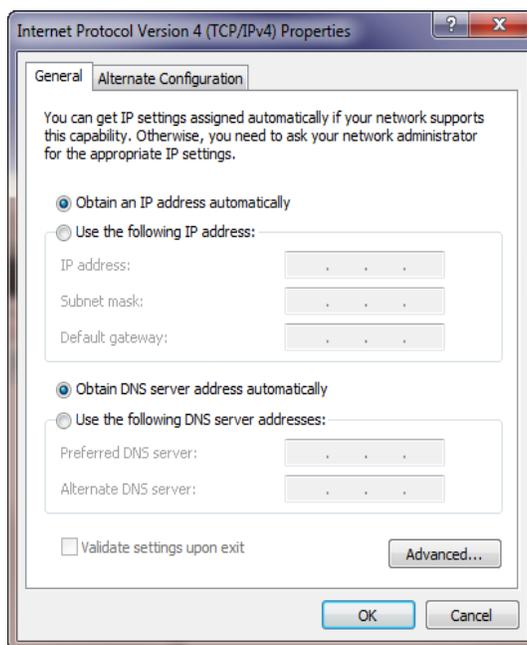
7. Select **Obtain an IP address automatically** and **Obtain DNS server address automatically**.
