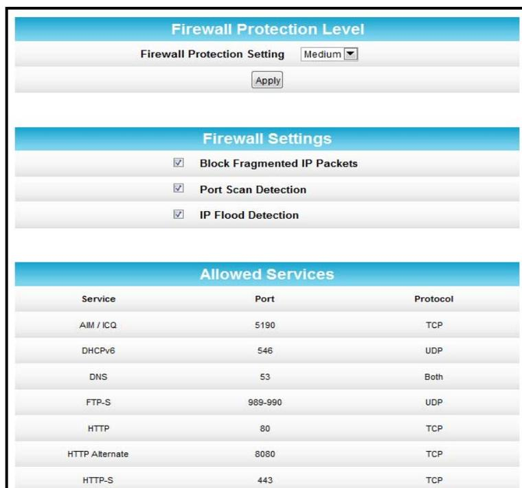
**Figure 28 – Firewall Protection Level Screen**
