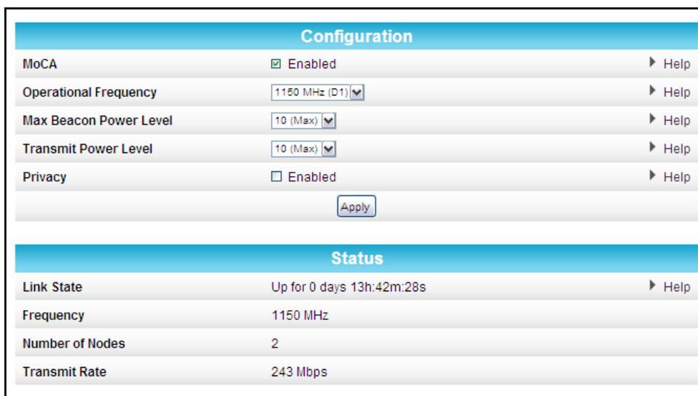
**Figure 27 – Basic MoCA Configuration and Status Screen**
