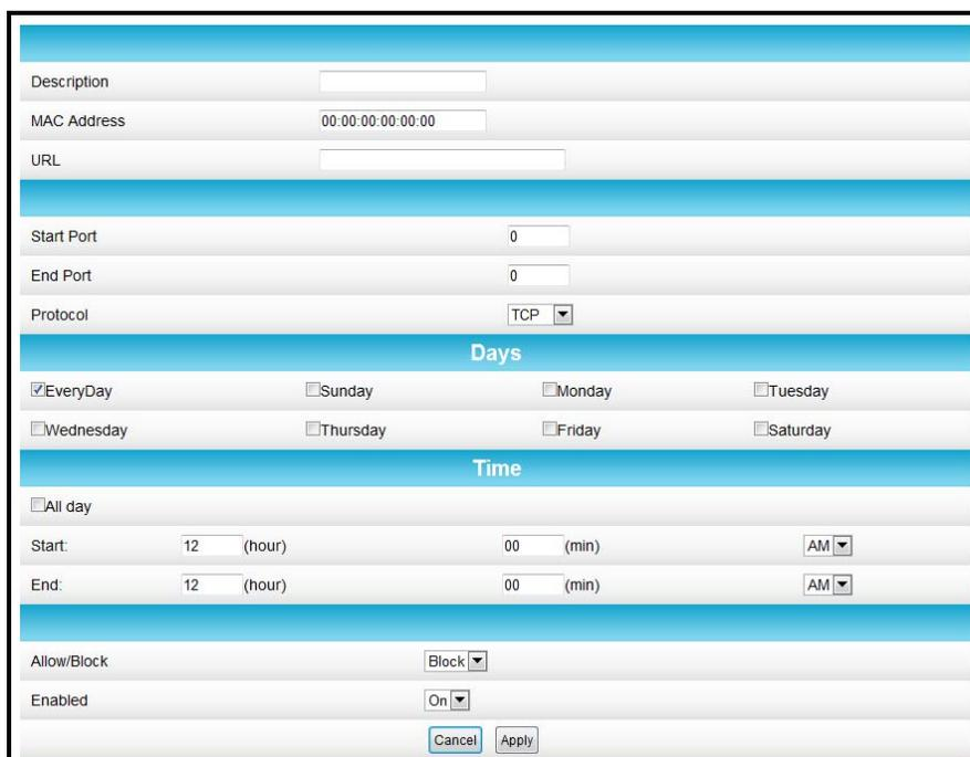
**Figure 19 – Firewall Parental Control Screen**
