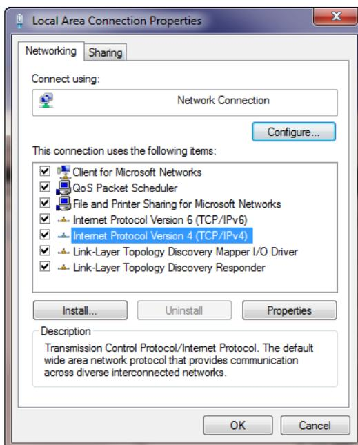
6. Select **Internet Protocol Version 4 (TCP/IPv4)** and then click **Properties** to open the TCP/IPv4 Properties window.
