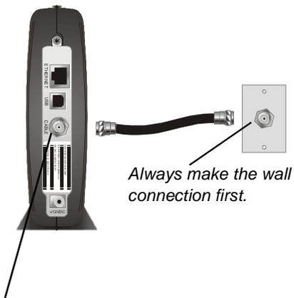
Before you connect or disconnect the USB or Ethernet cable, *always touch the coaxial cable connector on the cable modem.*
