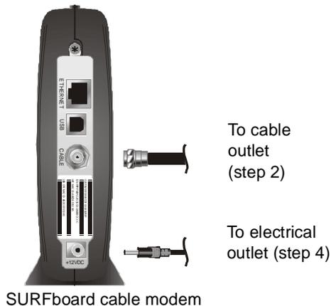
*Always connect coaxial cable to the wall outlet first.*
