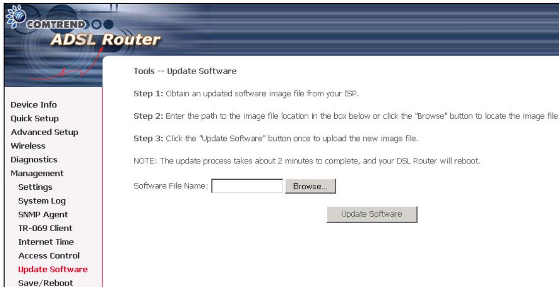
The screenshot shows the Comtrend ADSL Router web interface. On the left is a navigation menu with the following items: Device Info, Quick Setup, Advanced Setup, Wireless, Diagnostics, Management, Settings, System Log, SNMP Agent, TR-069 Client, Internet Time, Access Control, **Update Software** (highlighted in red), and Save/Reboot. The main content area is titled 'Tools -- Update Software' and contains the following text:
