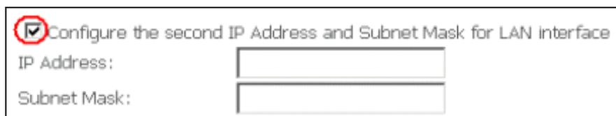
This close-up shows the checkbox 'Configure the second IP Address and Subnet Mask for LAN interface' which is checked. Below it are two empty input fields for 'IP Address:' and 'Subnet Mask:'.
