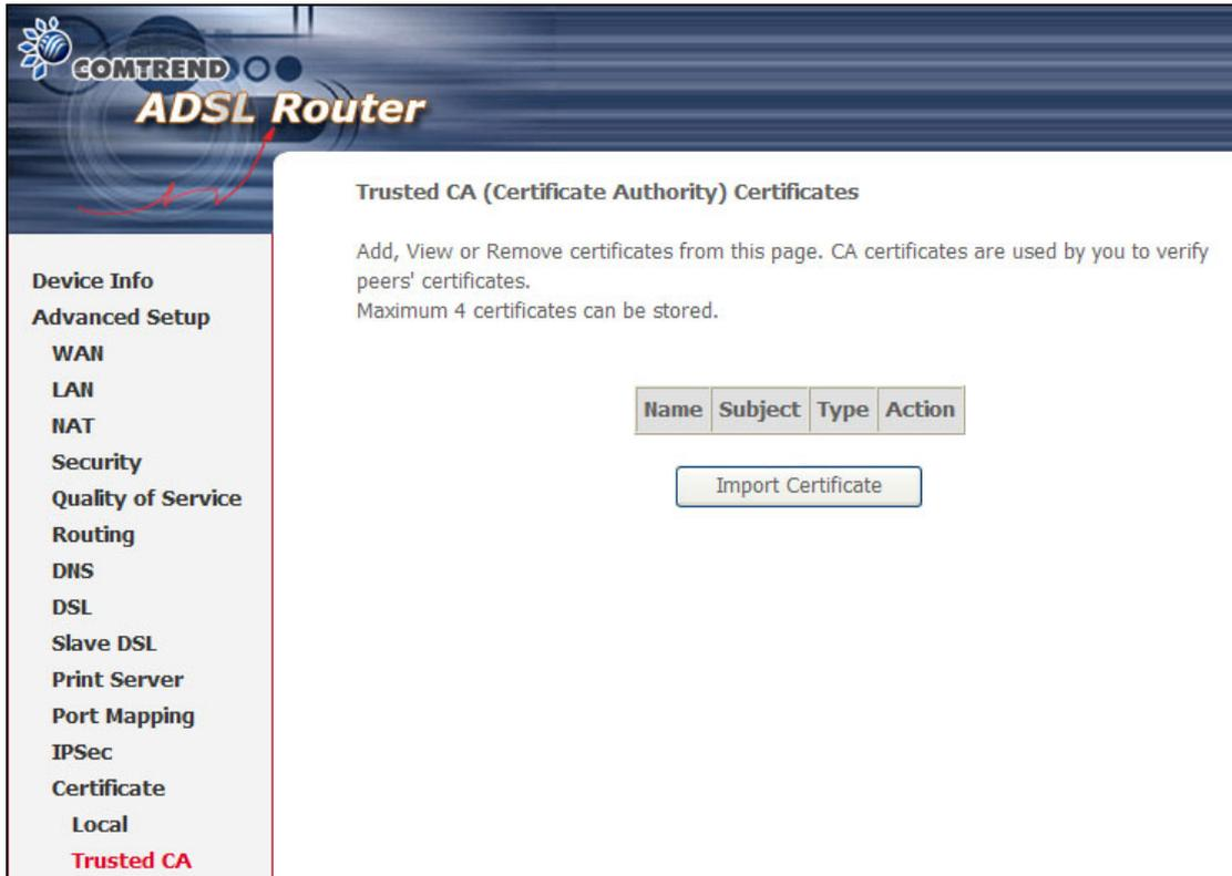
Click **Import Certificate** to paste the certificate content of your trusted CA. Generally speaking, the certificate content will be provided by your vendor/ISP/ITSP and is used to authenticate the Auto-Configuration Server (ACS) that the CPE will connect to.
