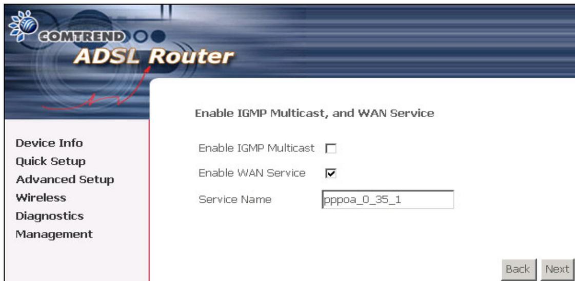
The screenshot shows the configuration interface for a Comtrend ADSL Router. The title bar at the top left features the Comtrend logo and the text "ADSL Router". A navigation menu on the left side includes the following items: "Device Info", "Quick Setup", "Advanced Setup", "Wireless", "Diagnostics", and "Management". The main content area is titled "Enable IGMP Multicast, and WAN Service" and contains the following settings:
