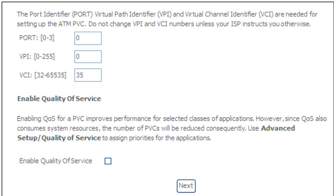
The Port Identifier (PORT) Virtual Path Identifier (VPI) and Virtual Channel Identifier (VCI) are needed for setting up the ATM PVC. Do not change VPI and VCI numbers unless your ISP instructs you otherwise.
