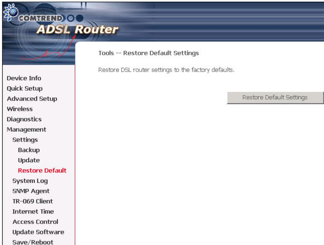
**NOTE 1:** This entry has the same effect as the hardware reset-to-default button. The device board hardware and the boot loader support the **reset to default** button. If the reset button is continuously pushed for more than 5 seconds, the boot loader will erase the entire configuration data saved on the flash memory.
