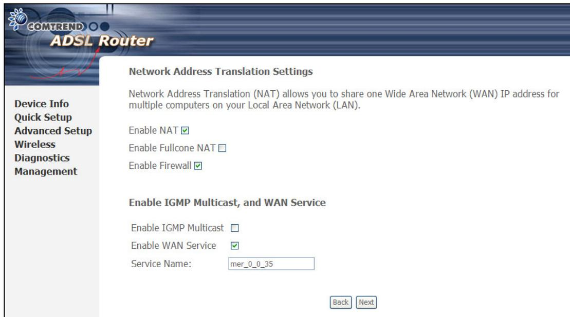
The screenshot shows the 'Network Address Translation Settings' page for a COMTREND ADSL Router. The page has a dark blue header with the COMTREND logo and 'ADSL Router' text. On the left, there is a navigation menu with options: Device Info, Quick Setup, Advanced Setup, Wireless, Diagnostics, and Management. The main content area is white and contains the following settings:
