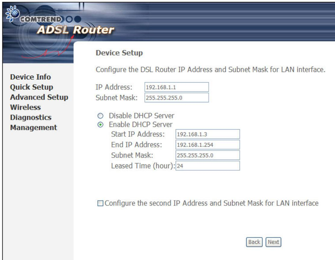
The screenshot shows the 'Device Setup' page for a COMTREND ADSL Router. The page has a dark blue header with the COMTREND logo and 'ADSL Router' text. On the left is a navigation menu with options: Device Info, Quick Setup, Advanced Setup, Wireless, Diagnostics, and Management. The main content area is titled 'Device Setup' and contains the following fields and options:
