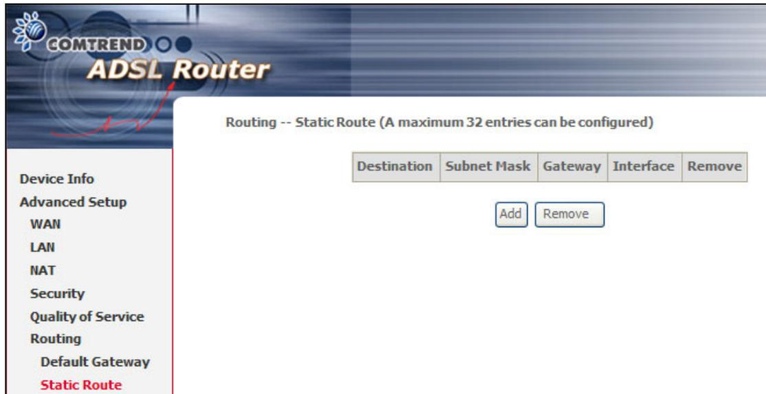
To add static route, click the **Add** button to display the following screen. Enter the destination network address, subnet mask, gateway AND/OR available WAN interface then click **Save/Apply** to add the entry to the routing table.
