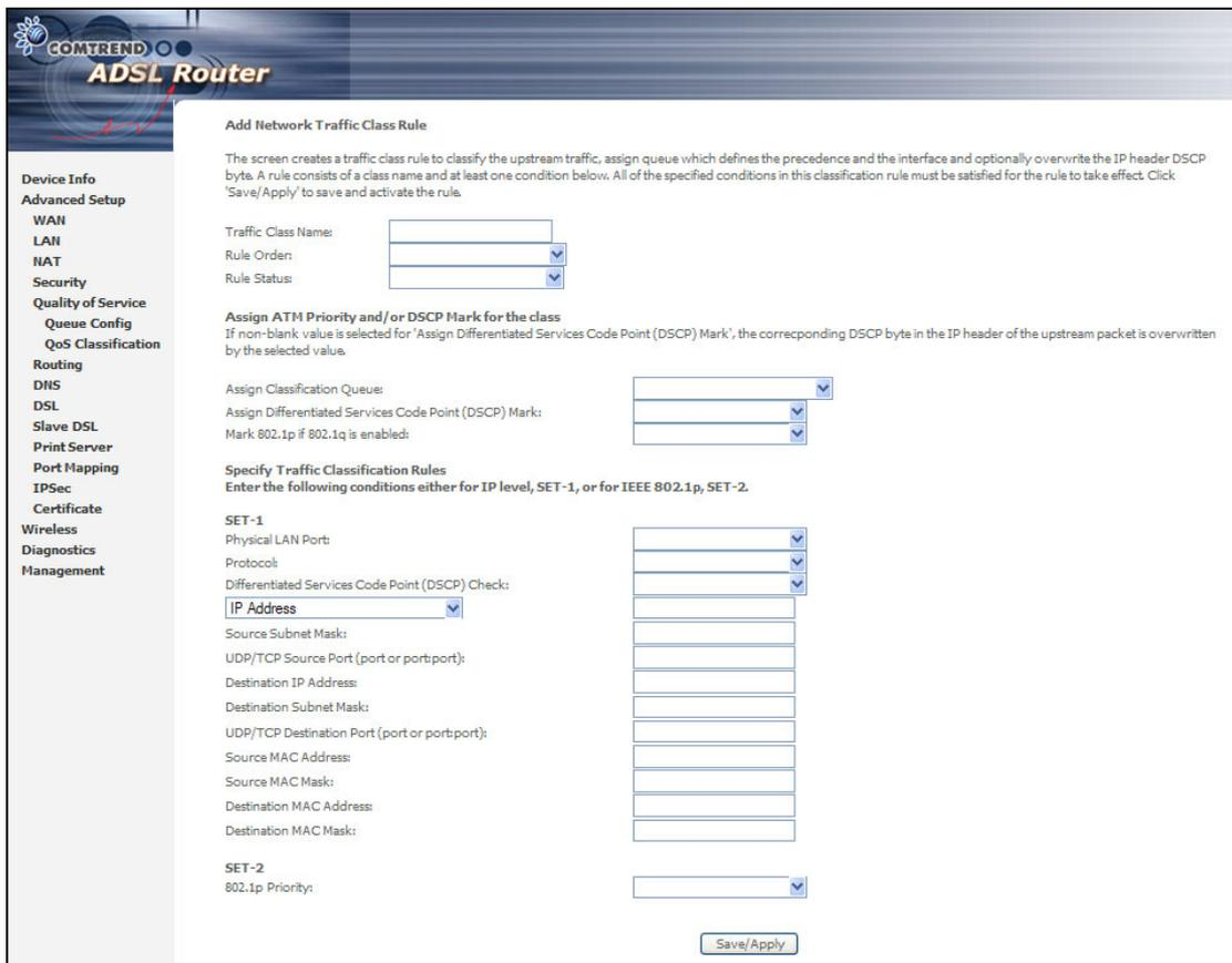
This screen creates a traffic class rule to classify the upstream traffic, assign queuing priority and optionally overwrite the IP header TOS byte. A rule consists of a class name and at least one condition below. All of the specified conditions in this classification rule must be satisfied for the rule to take effect.
