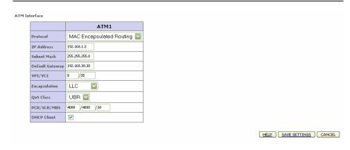
TABLE 6 List of parameters on MAC Encapsulated Routing ATM Interface
