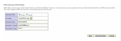
Upon DDNS Service Provider account creation, check the *Enable* radio button, choose the Provider name from the *Provider* list box and fill properly the *Domain Name*, the *Account / E-mail* and *Password / Key* fields.
