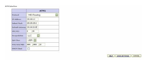
TABLE 4 List of parameters on 1483 Routing ATM Interface
