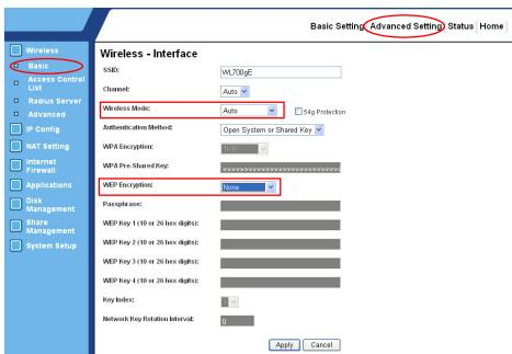
5. To enable encryption protection, set **Authentication** method to WEP 64-bits, WEP 128-bits, or WPA. For WEP encryption, you need to input four WEP keys (10 hexadecimal digits for WEP-64bits; 26 digits for WEP-128bits). You can also let the system generate the WEP keys by inputting a **Passphrase**. Take down all keys and passphrase in your note.
