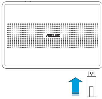
2. Wait for several seconds until the **READY** LED indicator flashes slowly. Press the **COPY** button on the front panel and the LED flashes quickly. This means WL-700gE is copying data from your USB storage. When the LED stops flashing and stays ON, it means data duplication is complete.
