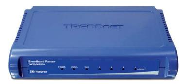
4-Port 10/100Mbps Ethernet Broadband Router Front Panel
