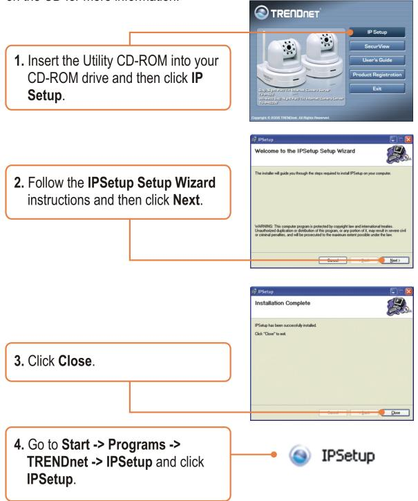
**Note:** By default, the IP setting on the TV-IP422/TV-IP422W is set to DHCP. Please skip to step 9. If you want to give the TV-IP422/TV-IP422W static IP address, continue on to step 5.
