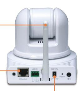
**3.** Connect the AC Power Adapter to the **Internet Camera Server** and then to a power outlet.
