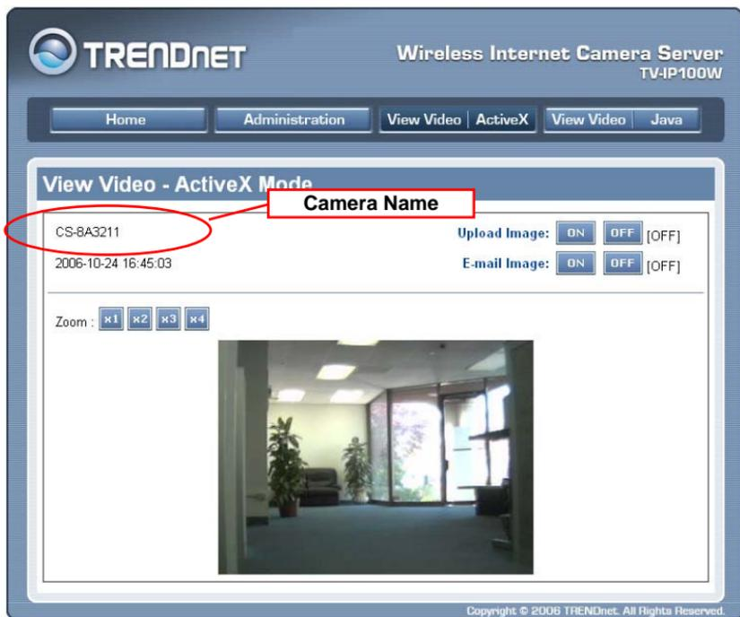
**Camera Name:** The Camera name will be displayed when the Camera Name field is entered in the Web Configuration setting under **Configuration**.
