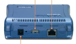
Connect the AC Power Adapter to the Print Server and then to a power outlet.
