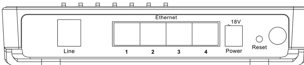
**Figure 1-4 Rear panel (4-port wireless model)**
