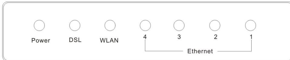
**Figure 1-2 Front panel (1-port and 4-port model))**
