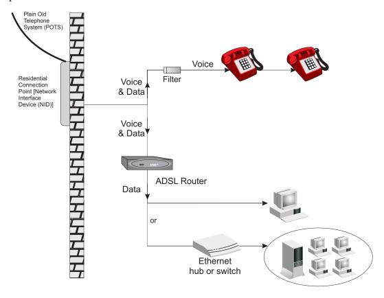
Figure 2-4. Installing without a Splitter
