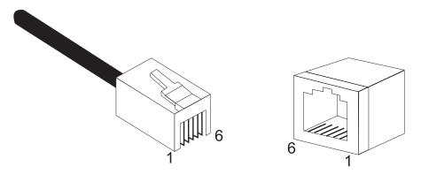
Figure B-2. RJ-11 Connector Pin Numbers
