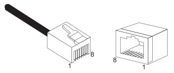
Figure B-1. RJ-45 Ethernet Connector Pin Numbers
