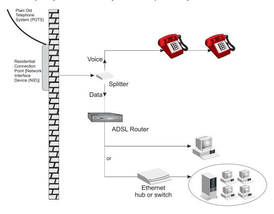
Figure 2-3. Installing with a Splitter
