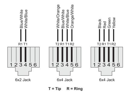
Figure B-3. RJ-11 Pinouts
