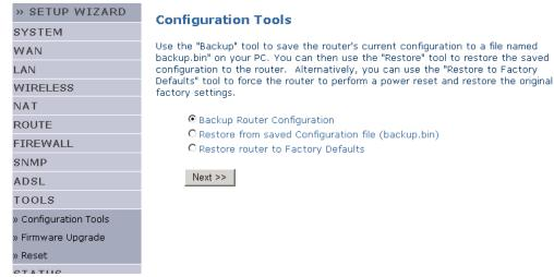
Backup allows you to save the ADSL Router's configuration to a file. Restore can be used to restore the saved backup configuration file. Restore to Factory Defaults resets the ADSL Router to the original settings.
