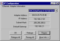
These values confirm that your ADSL Router is functioning. Click OK to close the IP Configuration window.
