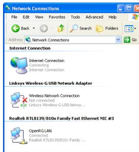
2. Double-click the wireless connection icon. The “Wireless Network Connection” screen appears, displaying all available wireless networks in the vicinity. If the FiOS Router is connected and active, the FiOS Router’s wireless connection is displayed. Note that the connection’s status is “Not connected” in the figure below.
