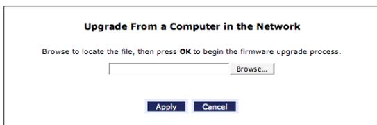
3. Enter the path of the software image file, or press the “Browse” button to browse for the file, and click **Apply**. Make sure to only use files with an “rmt” extension when performing the firmware upgrade procedure.
