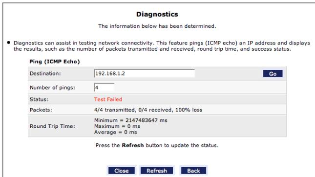
2. The FiOS Router automatically runs a ping test, and the results are displayed in the Diagnostics screen.
