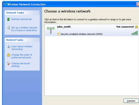
3. Click the connection once to mark it, then click **Connect** at the bottom of the screen. The following login window appears, asking for a “Network Key,” which is the pre-shared key used when configuring the FiOS Router’s WPA security (see the “WPA” section in this chapter).
