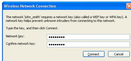
4. Enter the pre-shared key in both text boxes and click **Connect**. After the connection is established, its status will change to “Connected,” as shown below.
