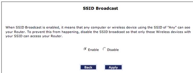
Click the “Enable” radio button to enable SSID broadcasting. If enabled, the SSID of the FiOS Router’s wireless network will be broadcast wirelessly. To disable SSID broadcasting, click the “Disable” radio button.
