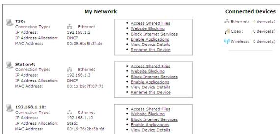
On the far right side of the screen, in the “Connected Devices” section, is list of the devices currently connected to the FiOS Router’s network, listed by connection type and number. The rest of the screen contains the “My Network” section, which displays each device connected to the FiOS Router’s network, and a series of basic configuration settings for each device.
