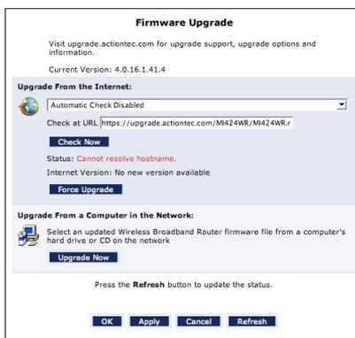
2. In the “Upgrade From a Computer in the Network” section, click **Upgrade Now**. The “Upgrade From a Computer in the Network” screen appears.
