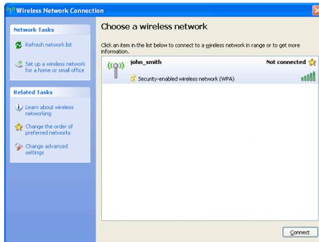
3. Click the connection once to mark it, then click **Connect** at the bottom of the screen. After the connection is established, its status will change to “Connected.”
