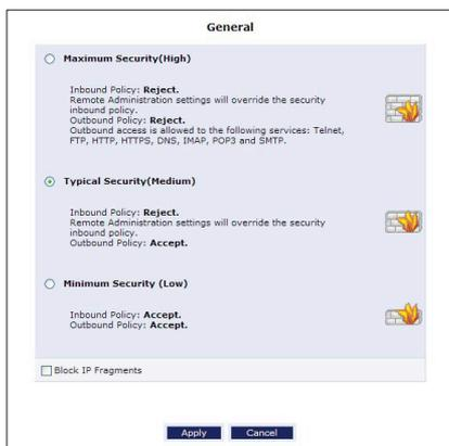
The FiOS Router features three pre-defined firewall security levels: **Maximum**, **Typical**, and **Minimum**. The table below summarizes the behavior of the FiOS Router for each of the three security levels.
