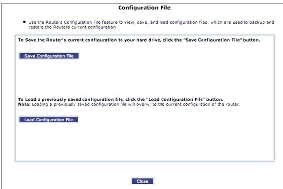
2. Click **Load Configuration File** to load the previous configuration from a file and restart the FiOS Router.
