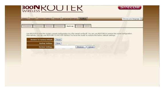
Use the "Backup" tool to save the Broadband router current configuration to a file named "**config.bin**" on your PC. You can then use the "Restore" tool to restore the saved configuration to the Broadband router. Alternatively, you can use the "Restore to Factory Defaults" tool to force the Broadband router to perform a power reset and restore the original factory settings.
