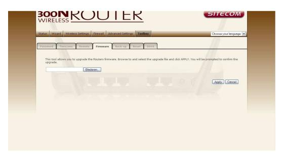
**Firmware Upgrade** This tool allows you to upgrade the Broadband router's system firmware. To upgrade the firmware of your Broadband router, you need to download the firmware file to your local hard disk, and enter that file name and path in the appropriate field on this page. You can also use the Browse button to find the firmware file on your PC.
