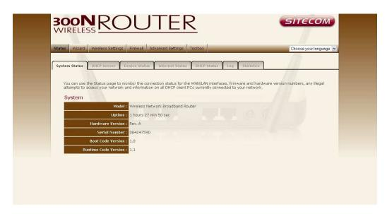
The System status section allows you to monitor the current status of your router the UP time, hardware information, serial number as well as firmware version information is displayed here.
