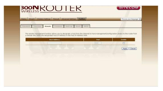
**Host Address** This is the IP address of the host in the Internet that will have management/configuration access to the Broadband router from a remote site. If the Host Address is left 0.0.0.0 this means anyone can access the router's web-based configuration from a remote location, providing they know the password.
