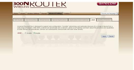
**UPnP Feature Disable** You can enable or Disable the UPnP feature here. After you enable the UPnP feature, all client systems that support UPnP, like Windows XP, can discover this router automatically and access the Internet through this router without having to configure anything. The NAT Traversal function provided by UPnP can let applications that support UPnP connect to the internet without having to configure the virtual server sections.
