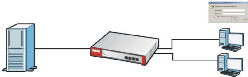
Figure 355 RADIUS Server Network Example
