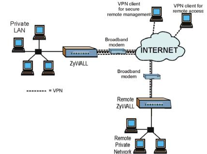
The following figure provides an example of a VPN application.
