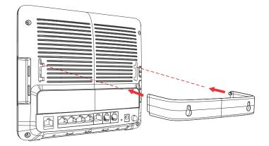
**5** Push the bracket up to tightly attach it to the Device.
