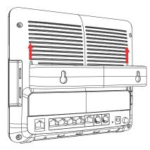
6 Mount the Device on the screws which are already installed on the wall. Make sure that the Device is firmly attached to the screws so it does not fall off.
