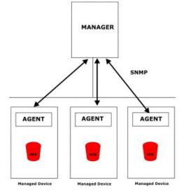
An SNMP managed network consists of two main types of component: agents and a manager.
