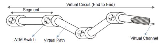
Think of a virtual path as a cable that contains a bundle of wires. The cable connects two points and wires within the cable provide individual circuits between the two points. In an ATM cell header, a VPI (Virtual Path Identifier) identifies a link formed by a virtual path; a VCI (Virtual Channel Identifier) identifies a channel within a virtual path. A series of virtual paths make up a virtual circuit.
