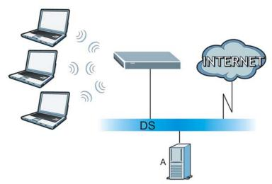
Figure 243 WPA(2) with RADIUS Application Example
