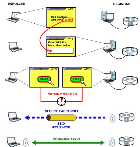
Figure 50 Example WPS Process: PIN Method
