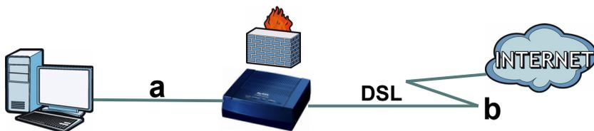
A computer can connect to the P-660R-T1 v3 using an Ethernet cable (a). The P-660R-T1 v3 then connects to the Internet (b), providing you with seamless access to the world's content.
