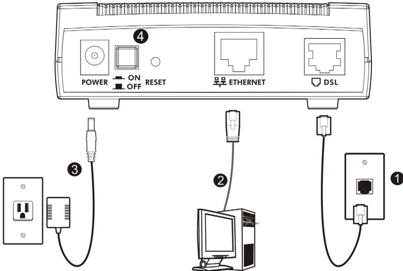
1. **DSL:** Use a telephone wire to connect this port to a telephone jack.
