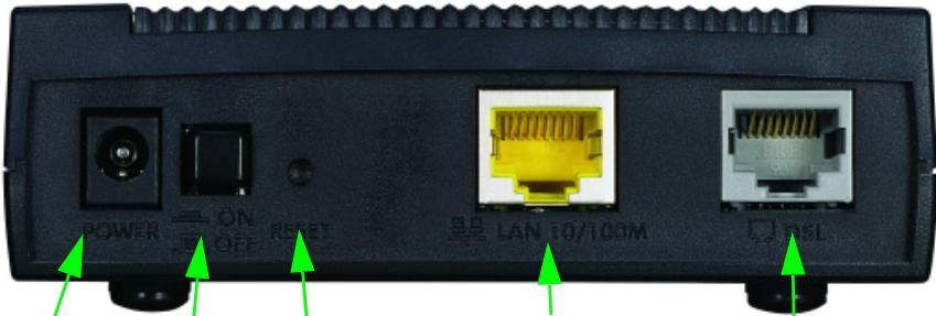
**POWER**      **ON/OFF**      **RESET**      **ETHERNET PORT**      **DSL PORT**
