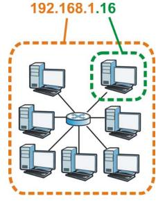
How much of the IP address is the network number and how much is the host ID varies according to the subnet mask.
