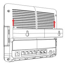
6 Mount the Device on the screws which are already installed on the wall. Make sure that the Device is firmly attached to the screws so it does not fall off.
