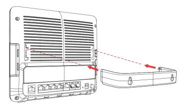
**5** Push the bracket up to tightly attach it to the Device.
