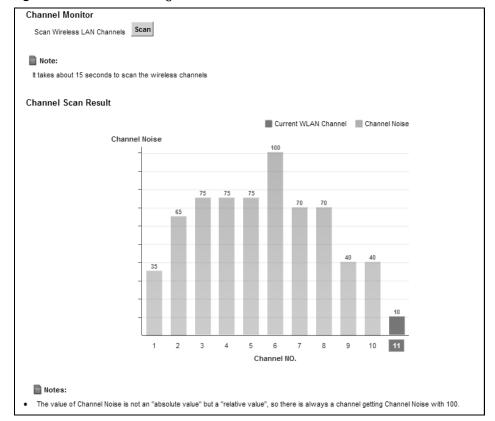
Figure 46 Network Setting > Wireless > Channel Status
