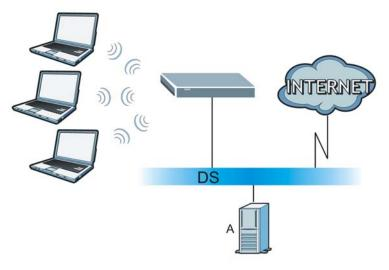
Figure 176 WPA(2) with RADIUS Application Example
