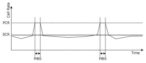
Figure 25 Example of Traffic Shaping
