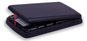
2 Insert your fingernail into the battery removal divot and lift the battery out of the battery compartment.
