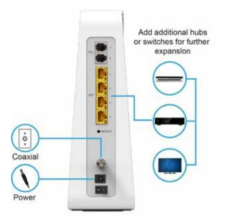
Sample Ethernet to Computer Connection (Connect Box model shown)
