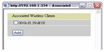
Associate Wireless Client displays a list of individual wireless device's MAC Address that are currently connected to the router.
