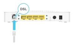
3 Plug the other end of the cable into the DSL/MODEM output port of your filter/splitter.
