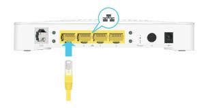
2 Connect the other end of the Ethernet cable to your network device.
