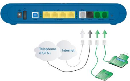
Use a phone cable with RJ-11 connectors to:
