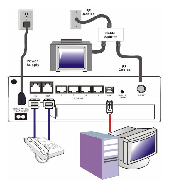
Fig. 2-2: USB Connection on DWG855
