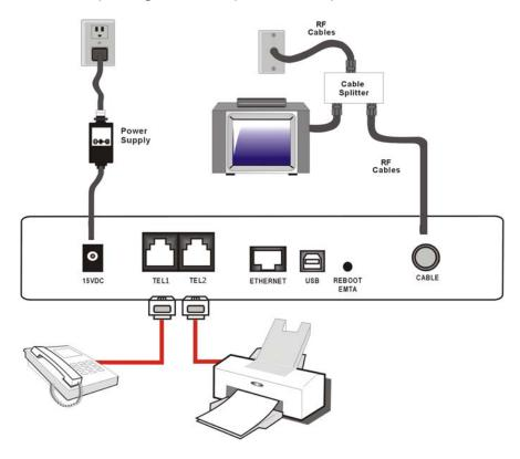
Fig. 5-1: Phone/Fax Connection on TWG850
