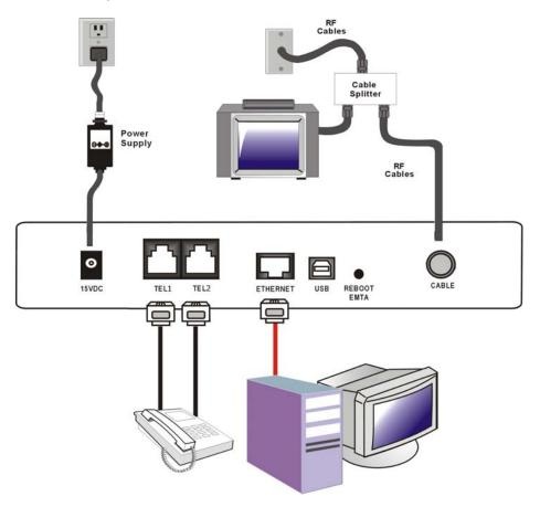
Fig.3-1: Ethernet Connection on TWG850
