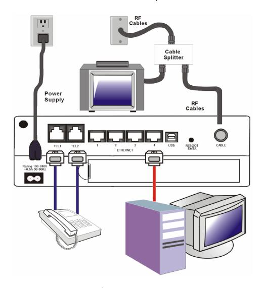
Fig.3-2: Ethernet Connection on DWG855
