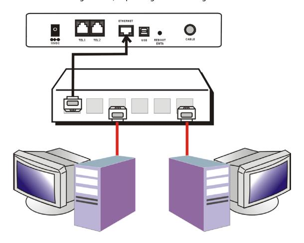
Fig.4-1: Hub Connection for TWG850
