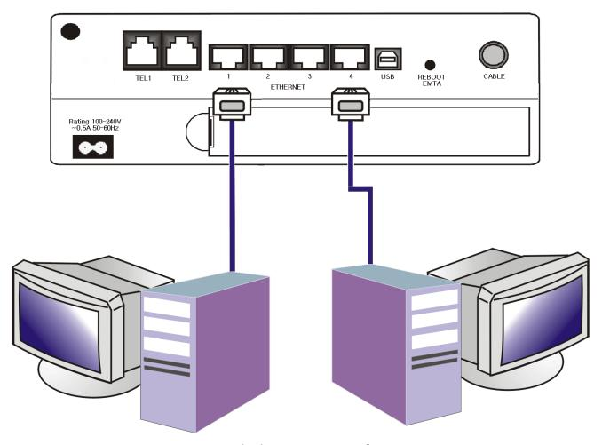
Fig.4-2: Multiple-PC Connection for DWG855
