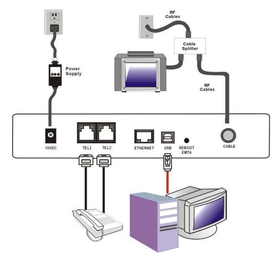
Fig. 2-1: USB Connection on TWG850
