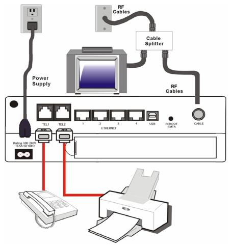
Fig. 5-2: Phone/Fax Connection on DWG855
