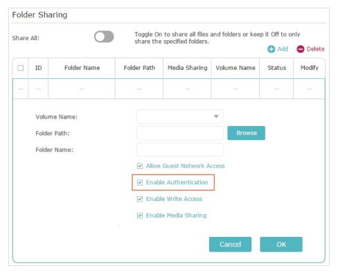
Note: Due to Windows credential mechanism, you might be unable to access the USB disk after changing Authentication settings. Please log out from the Windows and try to access again. Or you can change the address of the USB disk by referring to To Customize the Address of the USB Disk.
