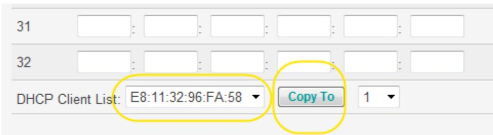
8. Alternatively, you can type the MAC address of the computer or device that you wish to allow access into the MAC address field:
