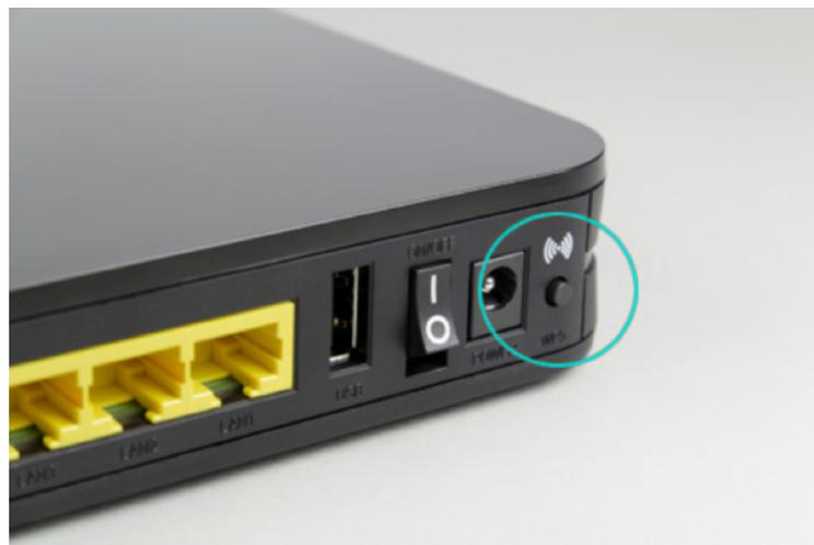
After pressing the WPS button briefly, the WPS light on the front of the router will flash slowly several times to indicate that the Intelligent wireless feature is re-checking for the best wireless channel to use.
