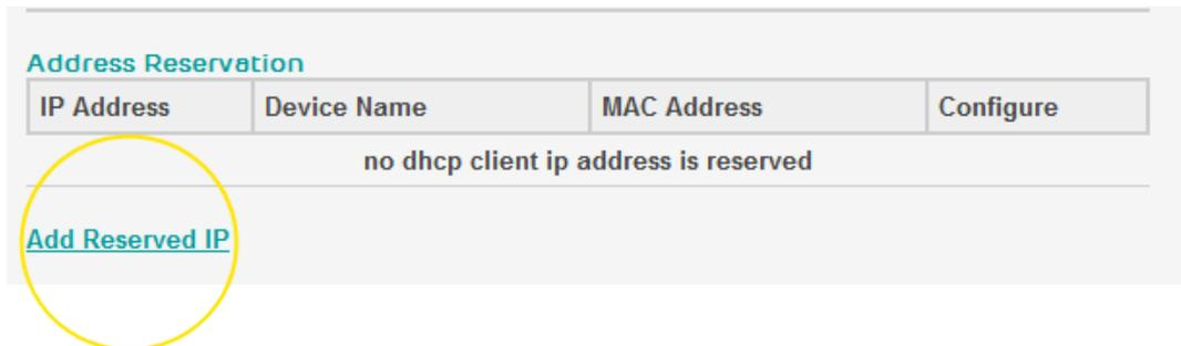
5. If the computer/device is already connected to the Bright Box, on the **DHCP client list** page, select the computer or device you wish to permanently assign the IP address to and click the **Add** link. You can identify the computer or device by the device name, or if no device name is available, by the MAC address of the device. In this example we are going to reserve the IP address for 'MyComputer':
