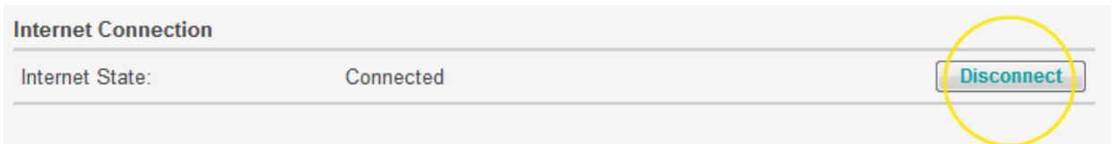
The 'Applying changes' message will be displayed, and the page will be displayed with the Internet State of 'Disconnected' visible. In the **Advanced Set-up > System > System Log** page the disconnected state appears as 'PPP connection down (VC1)'.
