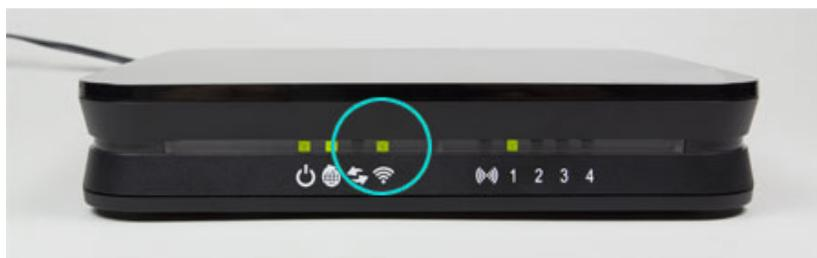
6. If the light is on or flickering, wireless is enabled. If the light is off wireless is disabled.
