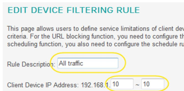
17. Select the type of traffic you want to block by ticking the 'blocking' box next to the service name. You can select multiple services to block, or block custom ports in the 'user define service' section. In this example we will block 'TCP' and 'UDP' (i.e. all traffic):
