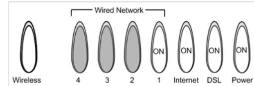
Note that a different Ethernet status light may be on, depending on which port you plug your cable into. If for any reason a connection is not made, double check that your broadband username and password have been typed in correctly.
