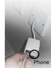
1) Plug one of the provided microfilters into your telephone socket. Any devices that were attached should then be plugged into the "Phone" socket of the microfilter.
