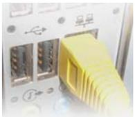
2) Plug the other end of the Ethernet cable into your computer's Ethernet port. This is often marked with the
