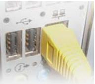
2) Plug the other end of the Ethernet cable into your computer's Ethernet port. This is often marked with the
