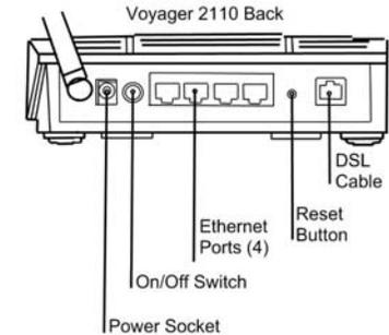
3) Plug one end of the grey DSL cable into the DSL socket on the back of the router, plug the other end into the microfilter (attached to your phone line in step 1). The microfilter socket is also marked DSL.
