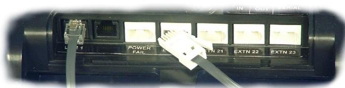
2. Plug the ADSL cable (purple) into the DSL socket on the back of the BT Micro. (Marked in purple)
