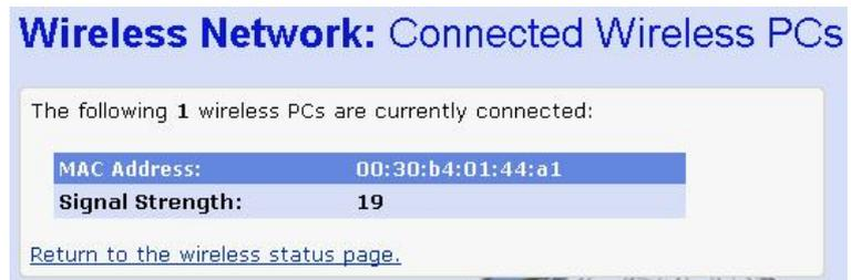
This page displays the MAC address of the PC currently connected to your BT Micro, together with the signal strength. The signal strength is the measure of radio frequency (RF) energy detected by the BT Micro on a specific channel. Signal strength may vary depending on the position of the PC(s) in relation to the BT Micro.
