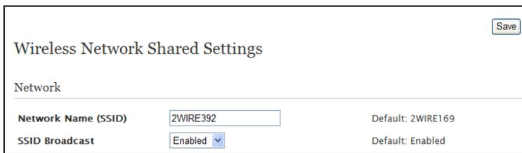
4. Enter a name assigned to your wireless network in the **Network Name (SSID)** field.
