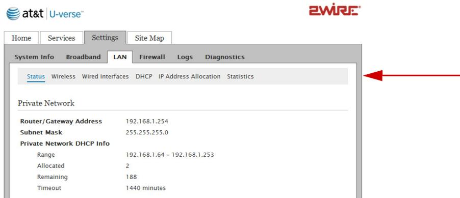
The screenshot shows the AT&T U-verse eWIRE interface. The top navigation bar includes 'Home', 'Services', 'Settings', and 'Site Map'. Below this, there are tabs for 'System Info', 'Broadband', 'LAN', 'Firewall', 'Logs', and 'Diagnostics'. The 'LAN' tab is selected, and a sub-menu is open showing 'Status', 'Wireless', 'Wired Interfaces', 'DHCP', 'IP Address Allocation', and 'Statistics'. A red arrow points to the 'Statistics' link. The main content area displays 'Private Network' information:
