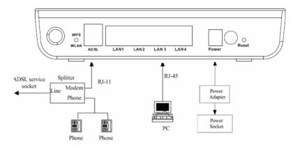
Figure 1 Connection diagram (Without connecting telephone sets before the splitter)
