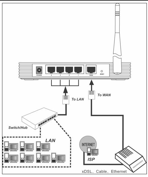
Figure 2-3 Hardware Installation of the Router
