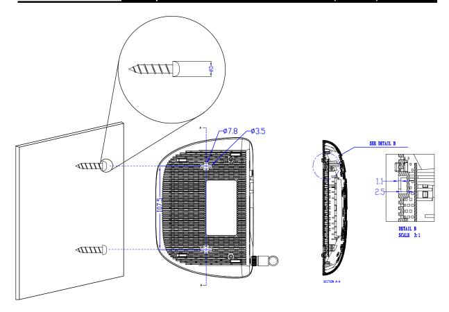
Figure 2-3 Wall-mount Install
