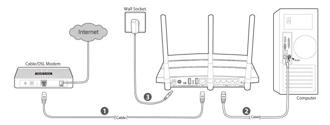
Figure 2-1 Hardware Installation
