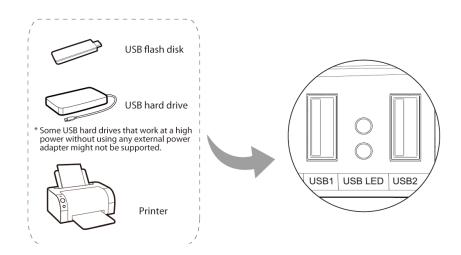
Figure 2-2 USB Installation
