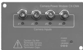
The camera module is designed expressly for use with UStec indoor and outdoor surveillance cameras. It is capable of powering up to 4 cameras. Power is supplied to the cameras from the UX-DC6.2 low voltage power supply, through the RG6 coaxial cable, to connectors on the rear of the camera module. The coaxial cable inputs from the cameras connect to the face of the camera module. The output from the camera module connects to the internal port on the internal CX amplifier.
