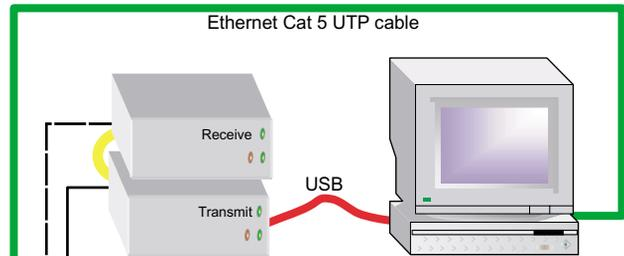
The transmit and receive units are interconnected. The interconnected units are connected to the PC running a Windows  $\mu$  operating system via a USB cable
