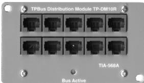
The TP-DM10R is a 10 port RJ45 distribution module that replaced the TP-DM6R module (shown on next page). In addition to having four more RJ-45 ports, the unit is wired in parallel, allowing it to operate on its own, without the need for ribbon cables and a TP-IN4 module.
