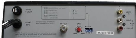
This particular modulator is a mono modulator, which means that the left and right audio signals get mixed together. UStec offers stereo versions if you are
