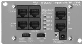
The TP-IN4RS is a telephone line interface and surge suppression module. Connections are present for incoming CO lines, dial tone out to a KSU phone system, two RJ31X-enabled devices, and a Category 5 rated coupler.
