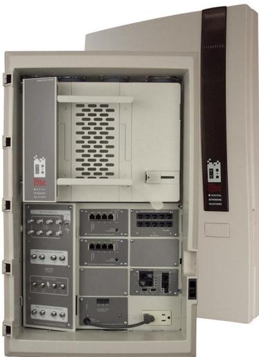
The flexible holster design is capable of handling a host of broadband devices from cable modem routers, xDSL routers, even third party servers.
