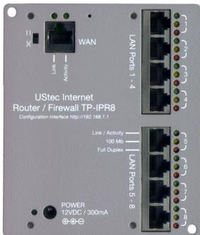
The TP-IPR8 is an 8 port switched router that is designed to share a high speed broadband connection for all the computers in the home. The unit also provides firewall security through network address translation.
