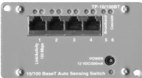
The TP-10/100BT Ethernet Switch replaces the TP-10BT Ethernet Hub.
