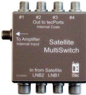
The CX-DSS4 is a dual LNB multiswitch for use with standard (non-HDTV) DSS dishes and receivers. It features dual LNB inputs, and four outputs for connection of up to four non-HDTV, DirecTV compatible tuners. The CX-DSS4 can be mounted in the UX-10x enclosure in two different places depending upon the panel module used
