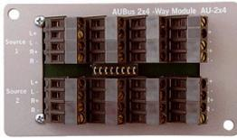
The AU-2X4 is a passive audio speaker distribution hub that consists of eight stereo wire connectors wired in parallel. The device can be set up in either of two ways:
