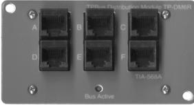
The TP-DM6R module has been discontinued but is shown here for reference. The TP-DM6R module provides telephone distribution to six rooms. When connected to the TP-IN4 module, these units distribute up to four telephone lines to six different locations. It is possible to distribute six KSU extensions to six locations in the home with the TP-KSU6R14 adapter cable, however the TP-KSU8 module and adapter cables replace the TP-DM6R/-KSU6R14 in new installations.
