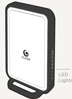
NOTE: The number of lights indicates the CLEAR 4G signal strength. For optimal signal strength, you should try different locations for the Modem to ensure a minimum of two lights are lit.
