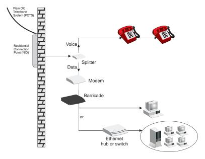
Figure 2-3. Installing with a Splitter
