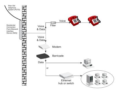
Figure 2-4. Installing without a Splitter
