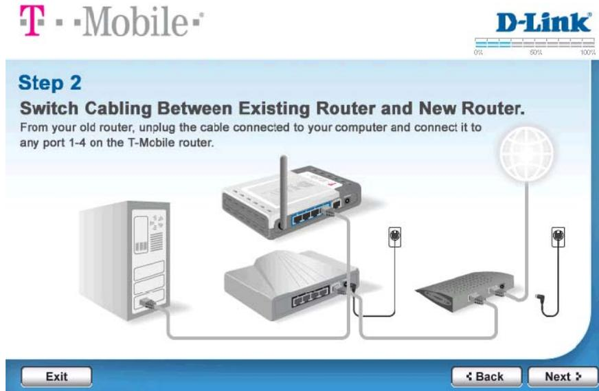
3. Unplug the cable connected to your modem from your old router and plug it into the TM-G5240's Internet port. When done, click the **Next** button on the Wizard.
