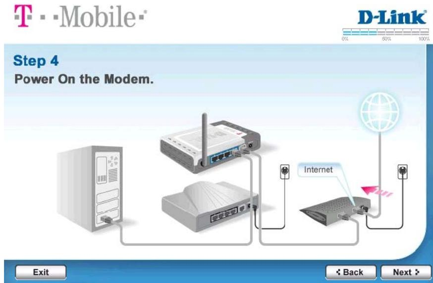
5. Plug the power adapter into the back of the TM-G5240. When done, click the **Next** button on the Wizard.
