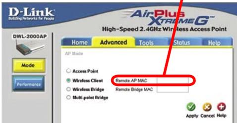
When using the DWL-2000AP in **Wireless Client** mode, you will enter the MAC address of the Remote AP.
