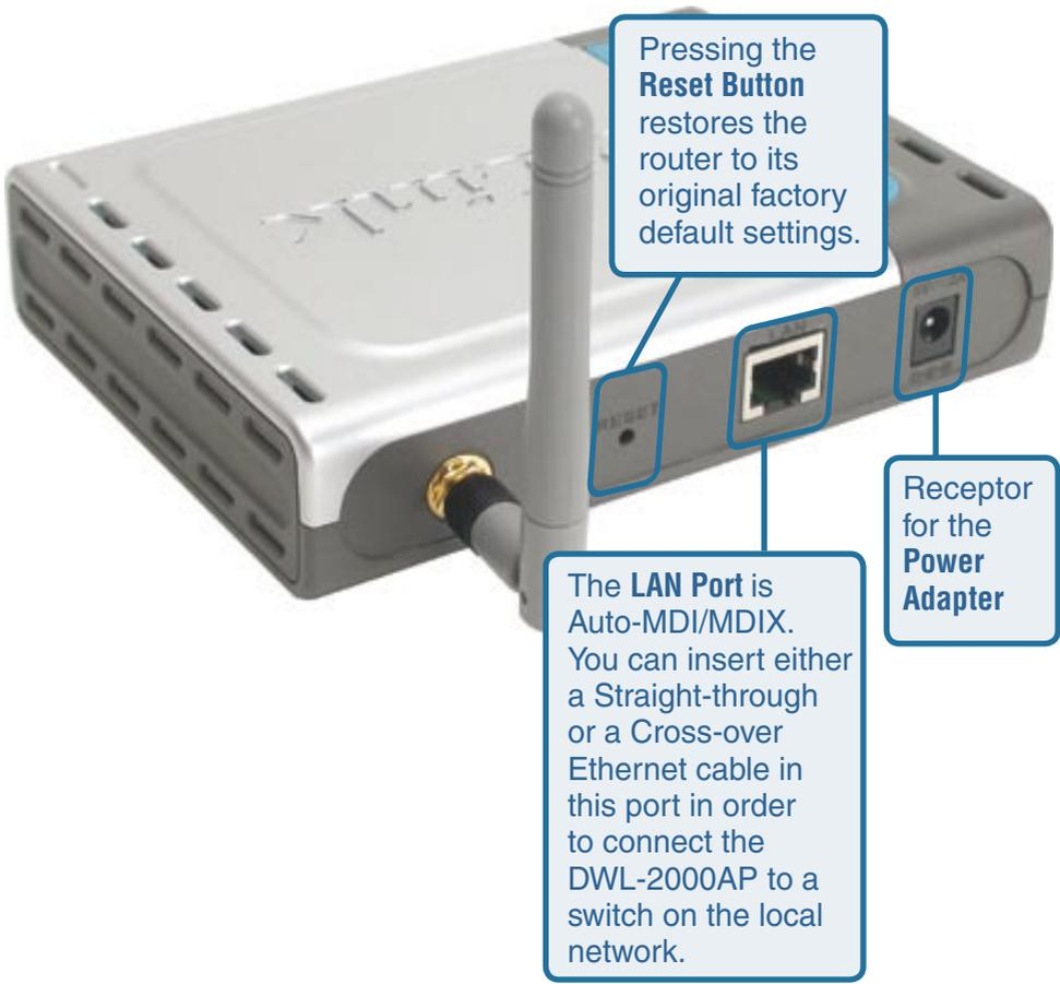
Pressing the **Reset Button** restores the router to its original factory default settings.
