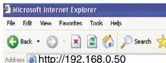
Note: if you have changed the default IP Address assigned to the DWL-2000AP, make sure to enter the correct IP Address.
