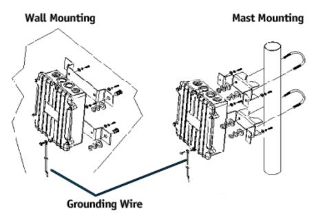
The DWL-1700AP can be mounted on the side of a building or mounted to a mast as shown in the picture above. A wall (side) mount allows for mounting the DWL-1700AP on the side of a building. This will provide a convenient mounting location when the roof overhang is not excessive and/or the location is high enough to provide a clear line of sight.
