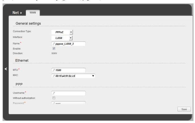
Figure 66. The page for creating a new connection. The **General settings** and **Ethernet** sections.
