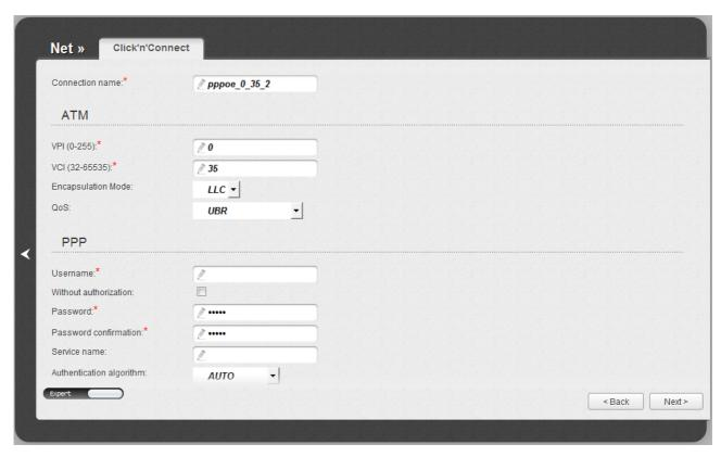
Figure 27. Configuring PPPoE WAN connection. The expert settings mode. The ATM section.
