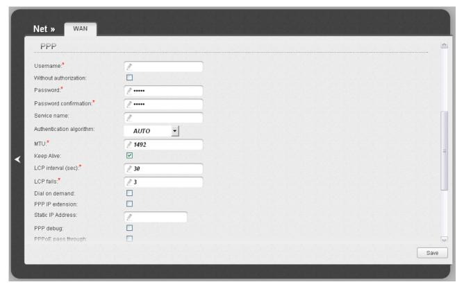
Figure 68. The page for creating a new connection. The **PPP** section.
