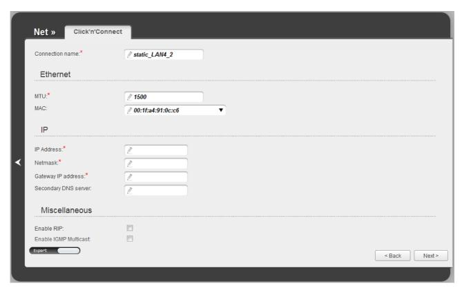
Figure 33. Configuring Static IP WAN connection. The expert settings mode. The **Ethernet** section.
