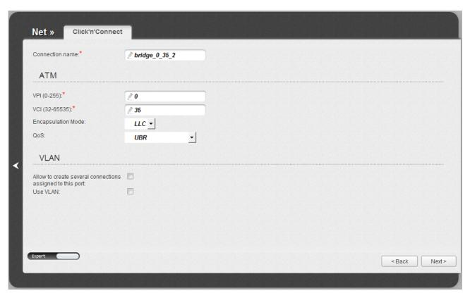
Figure 40. Configuring Bridge WAN connection. The expert settings mode. The ATM and VLAN sections.
