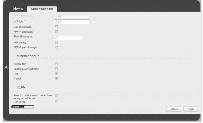
Figure 30. Configuring PPPoE WAN connection. The expert settings mode. The **Miscellaneous** and **VLAN** sections.
