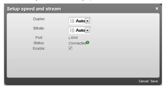
Figure 85. The page for changing parameters of the router's LAN port.
