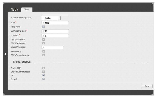
Figure 63. The page for creating a new connection. The Miscellaneous section.
