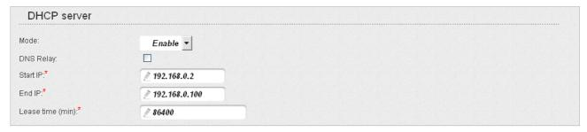
Figure 72. The section for configuring the DHCP server.
