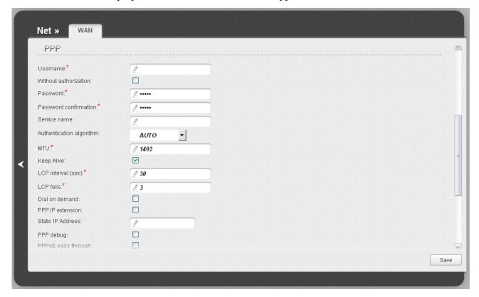
Figure 59. The page for creating a new connection. The **PPP** section.
