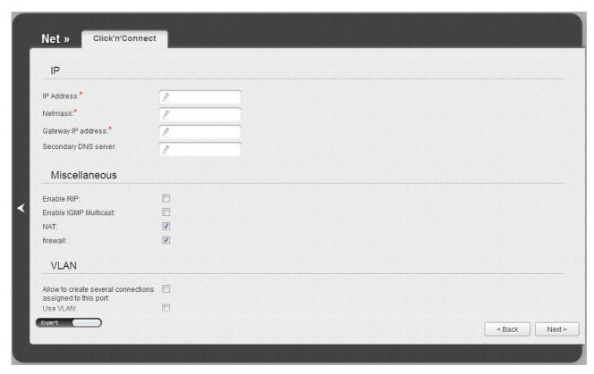
Figure 34. Configuring Static IP WAN connection. The expert settings mode. The **Miscellaneous** and **VLAN** sections.
