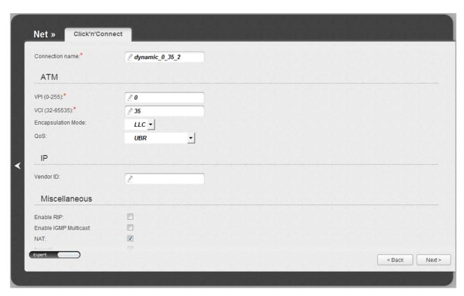
Figure 36. Configuring Dynamic IP WAN connection. The expert settings mode. The **ATM** and **IP** sections.
