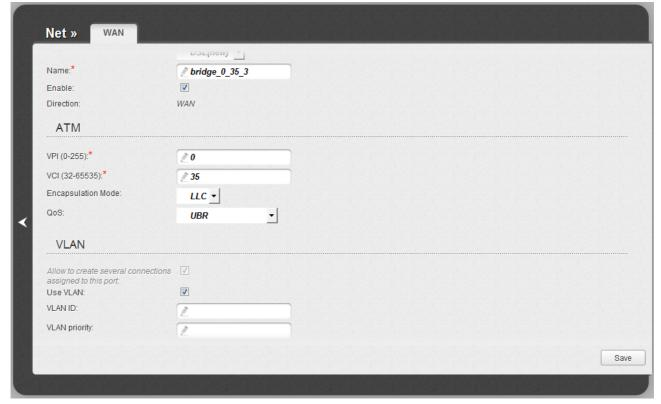
Figure 62. The page for creating a new connection. The **VLAN** section.
