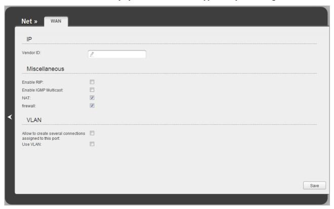
Figure 67. The page for creating a new connection. The Miscellaneous section.
