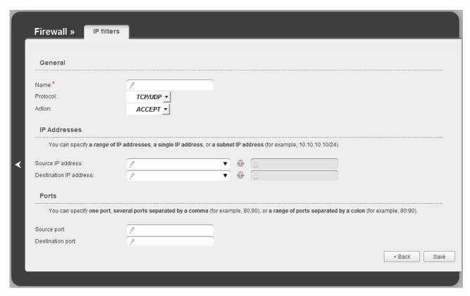
Figure 94. The page for adding a rule for IP filtering.
