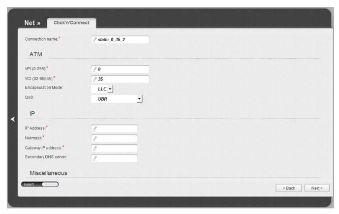
Figure 32. Configuring Static IP WAN connection. The expert settings mode. The ATM and IP sections.
