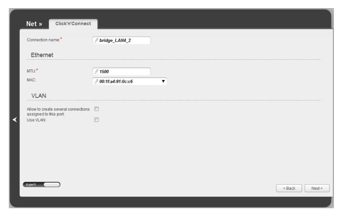
Figure 41. Configuring Bridge WAN connection. The expert settings mode. The **Ethernet** section.
