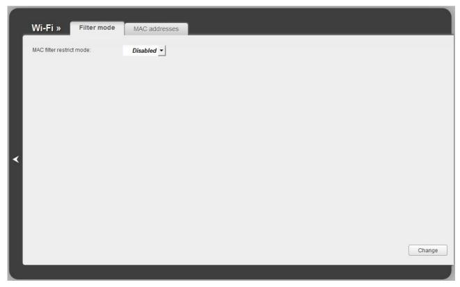
Figure 78. The MAC filter for the wireless network.
