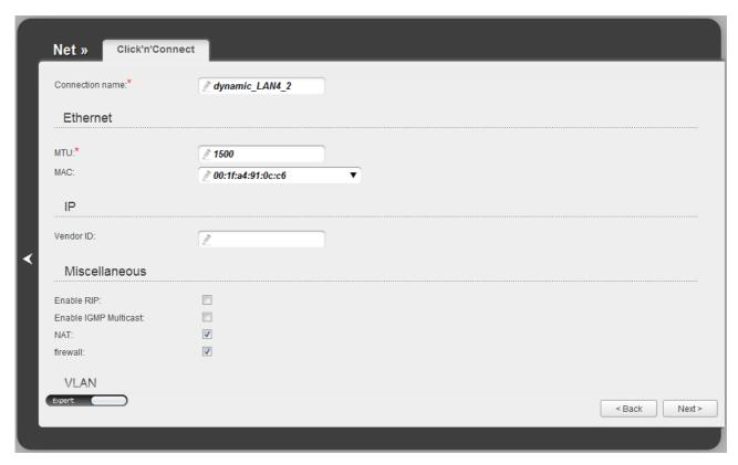
Figure 37. Configuring Dynamic IP WAN connection. The expert settings mode. The **Ethernet** section.
