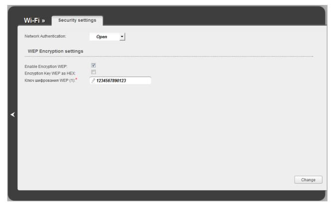
Figure 76. The Open value is selected from the Network Authentication drop-down list.
