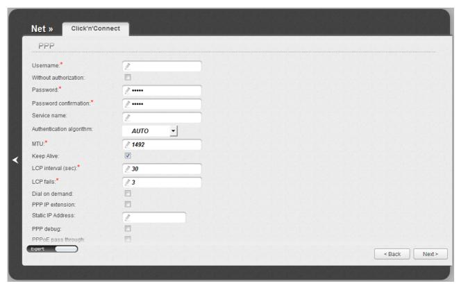
Figure 29. Configuring PPPoE WAN connection. The expert settings mode. The **PPP** section.
