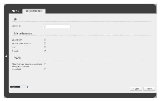
Figure 38. Configuring Dynamic IP WAN connection. The expert settings mode. The **Miscellaneous** and **VLAN** sections.
