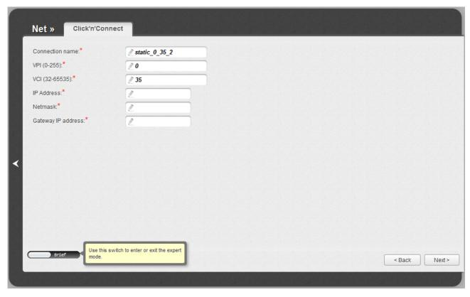
Figure 31. Configuring Static IP WAN connection.
