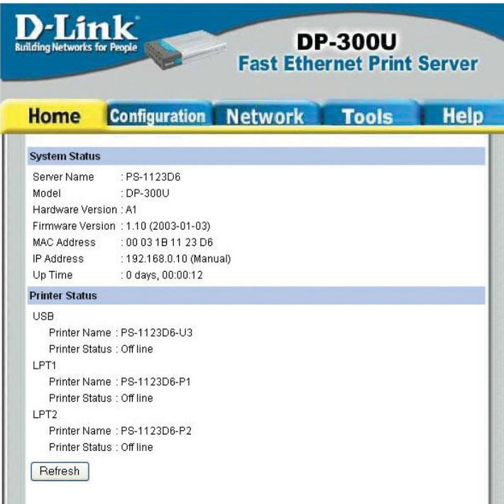
The screenshot shows the web interface for the D-Link DP-300U Fast Ethernet Print Server. The header includes the D-Link logo and the product name. A navigation menu has tabs for "Home", "Configuration", "Network", "Tools", and "Help". The main content area is divided into two sections: "System Status" and "Printer Status".
