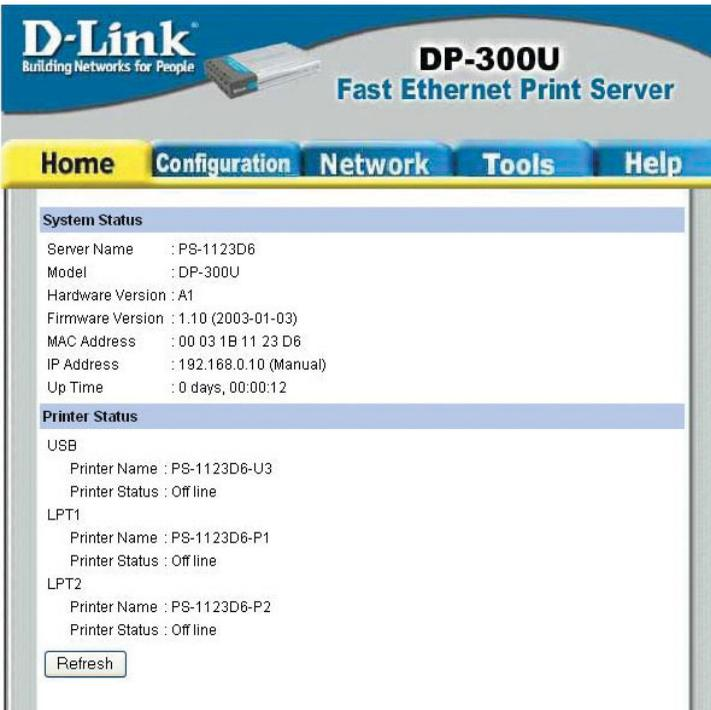
A screenshot of the D-Link DP-300U Fast Ethernet Print Server web interface. The header features the D-Link logo and the product name "DP-300U Fast Ethernet Print Server". A navigation menu includes "Home", "Configuration", "Network", "Tools", and "Help". The main content area is divided into two sections: "System Status" and "Printer Status".
