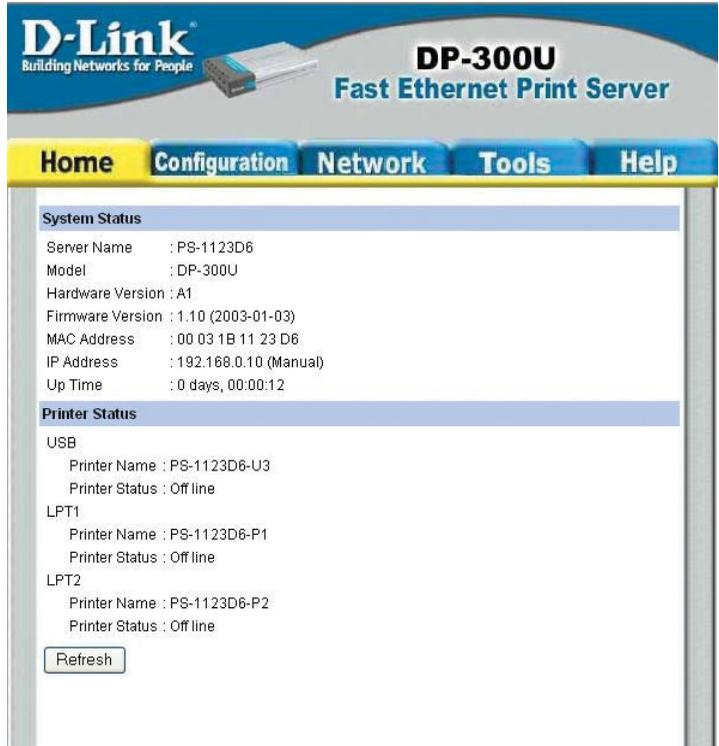
The screenshot shows the D-Link DP-300U Fast Ethernet Print Server web configuration interface. The 'System Status' tab is selected, displaying the following information:
