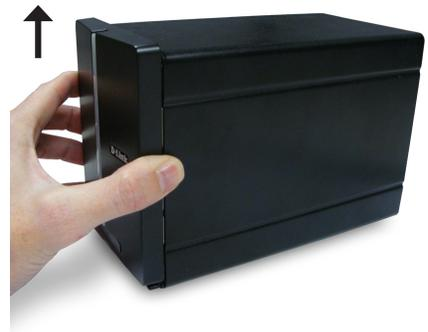
2. Once the faceplate is unlatched, pull it off the device, exposing the drive bays.
