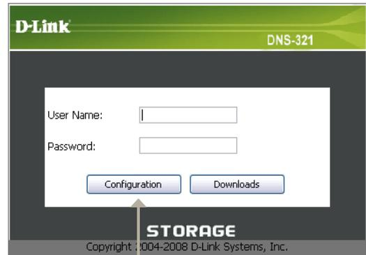
When logging into the DNS-321 for the first time, you will be asked to choose a drive configuration type and format the drives. There are four options: **Standard**, **JBOD**, **RAID 0** and **RAID 1**. Standard configures each disk as a separate volume, while JBOD combines both disks into a single volume. See page 47 for more details on using the RAID configurations.
