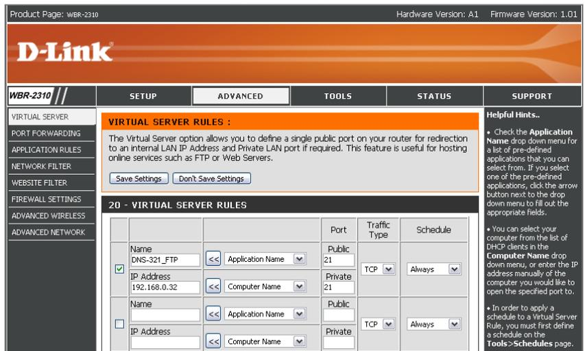
If you use an FTP port other than 21, then users accessing the FTP server using an FTP client will have to specify the non-standard port, and users who are using a browser will have to specify the port in the URL (e.g. ftp://ftp.dns321.com:3000, where the FTP port is 3000).
