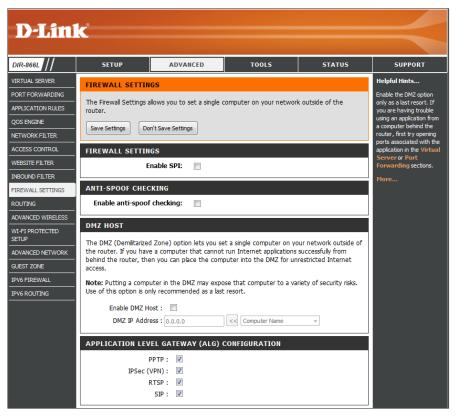
PPTP: Check the box to allow multiple machines on the LAN to connect to their corporate network using PPTP protocol.
