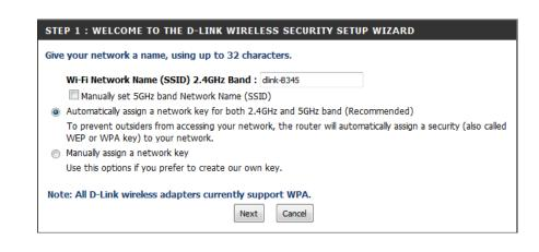
Enter a **Wi-Fi Network Name** for your 2.4GHz wireless networks (SSID). Do not use personal information as your SSID since users with wireless devices within range of your router will be able to see this information. Check the box to manually set the **Network Name** for the 5GHz band.
