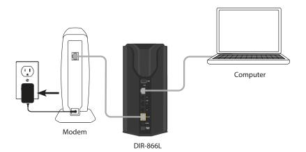
5. Plug the power adapter into your router and connect to an available power outlet or surge protector. If the Power LED does not light up, press the Power button on the back of the router.
