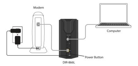
6. After the router has powered up, verify that the power (green) and Internet (orange or green) LEDs are both lit. Skip to "Configuration" on page 13 to learn about your configuration options.
