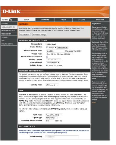
Visibility Status: Select Invisible if you do not want the SSID of your wireless network broadcasted by the DIR-866L. If Invisible is selected, the SSID of the DIR-866L will not be seen by Site Survey utilities so your wireless clients will have to know the SSID of your DIR-866L in order to connect to it.
