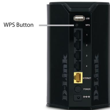
**Step 2** - Within 2 minutes, press the WPS button on your wireless client (or launch the software utility and start the WPS process).
