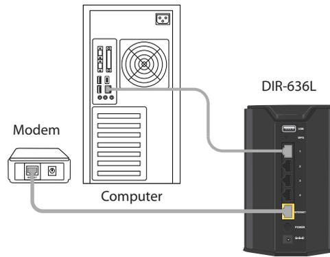
5. Reconnect the power adapter to your cable or DSL broadband modem and wait for two minutes.
