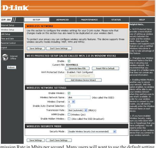
**Transmission** Use the drop-down menu to select the appropriate Transmission Rate in Mbits per second. Many users will want to use the default setting, **Rate:** *Best (automatic)*.
