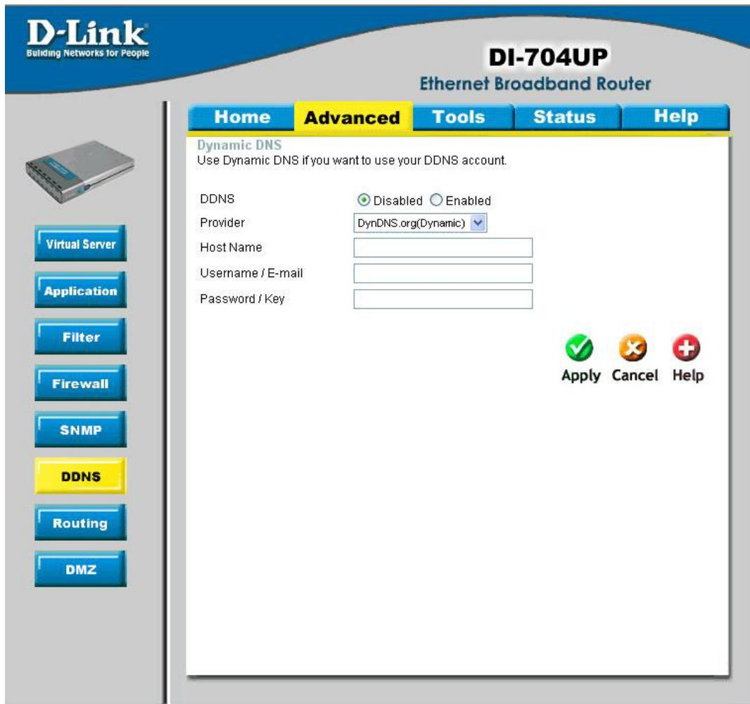
DDNS (Dynamic Domain Name System) keeps dynamic IP addresses (e.g., IP addresses assigned by a DHCP capable router or server) linked to a domain name. Users who have a Dynamic DNS account may use this feature on the DI-704UP.
