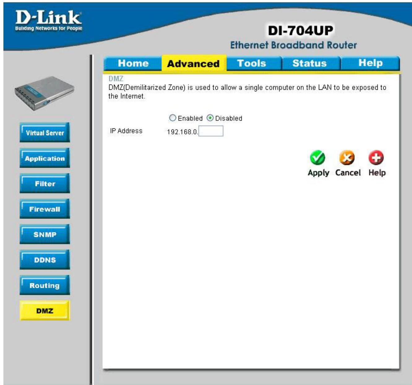
If you have a computer that cannot run Internet applications properly from behind the DI-704UP, then you can allow that computer to have unrestricted Internet access. Enable this feature and enter the IP address of that computer as a DMZ (Demilitarized Zone) host with unrestricted Internet access. Adding a client to the DMZ may expose that computer to a variety of security risks; so only use this option as a last resort.
