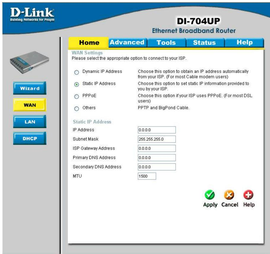
Choose Static IP Address if all WAN IP information is provided to you by your ISP. You will need to enter in the IP Address, subnet mask, gateway address, and DNS address(es) provided to you by your ISP. Each IP address entered in the fields must be in the appropriate IP form, which are four IP octets separated by a dot (x.x.x.x). The Router will not accept the IP Address if it is not in this format.
