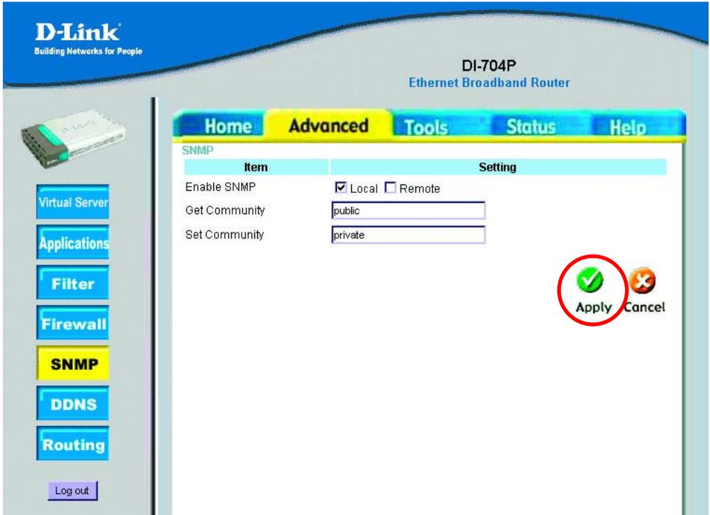
In brief, SNMP, the Simple Network Management Protocol, is a protocol designed to give a user the capability to remotely manage a computer network by polling and setting terminal values and monitoring network events.
