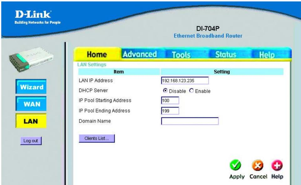
*LAN is short for Local Area Network. This is considered your internal network. These are the IP settings of the LAN interface for the DI-704P. These settings may be referred to as Private settings. You may change the LAN IP address if needed. The LAN IP address is private to your internal network and cannot be seen on the Internet.*
