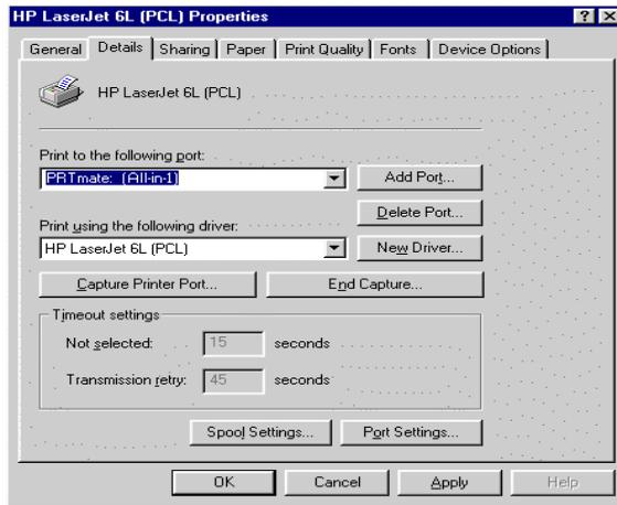
3. Choose the “PRTmate: (All-in-1)” from the list attached at the **Print To** item. Be sure that the **Printer Driver** item is configured to the correct driver of your *server printer*.
