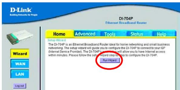
The **Setup Wizard** screen will appear. Follow the Wizard step by step to quickly configure the DI-704P.
