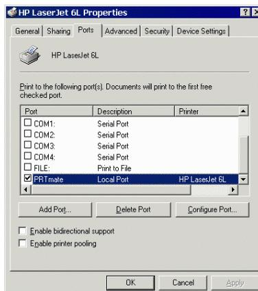
Compared to the procedure in last section, the selection of **Details** is equivalent to the selection of **Ports**, and **Port Settings** is equivalent to **Configure Port**.
