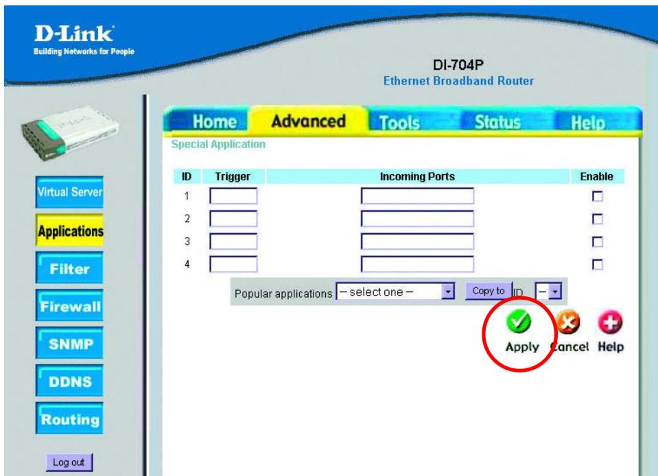
The screenshot displays the 'Special Application' configuration page on a D-Link DI-704P router. The page features a navigation bar with 'Home', 'Advanced', 'Tools', 'Status', and 'Help'. A sidebar on the left contains various configuration options: Virtual Server, Applications (highlighted), Filter, Firewall, SNMP, DDNS, and Routing, along with a 'Log out' button. The main content area contains a table for defining special applications:
