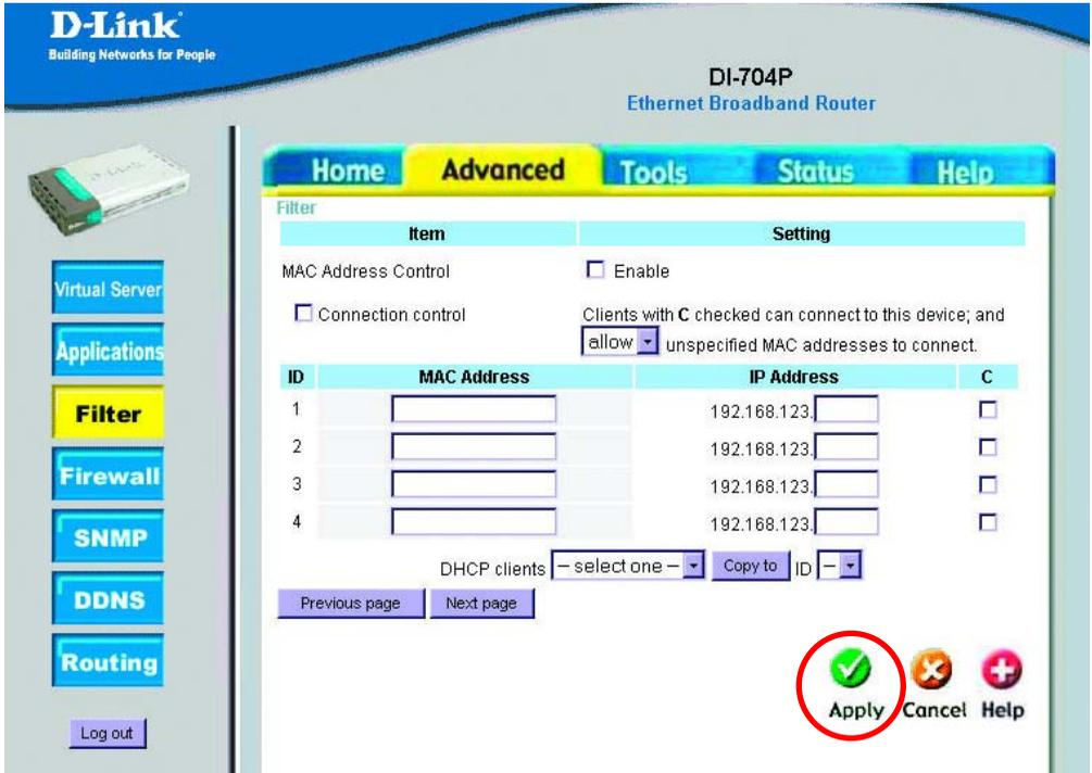
*MAC Address Control allows you to assign different access rights for different users and to assign a specific IP address to a certain MAC address.*
