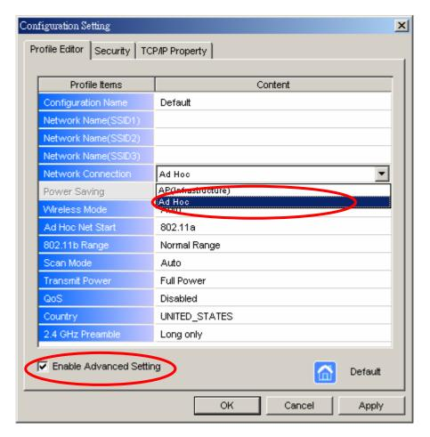
**NOTE!** Ad-hoc mode is available only for 802.11b/g. It is not available for 802.11a. This is a client product and do not have radar detection function specified by FCC. The software will not let you to use ad-hoc under 802.11a. The country domain can not be selected. It always shows "UNITED\_STATES".
