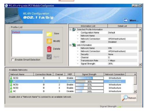
**Note!** To automatically connect to the network with the strongest signal, select **Enable Smart Selection**. **Any** displays in Profile List.
