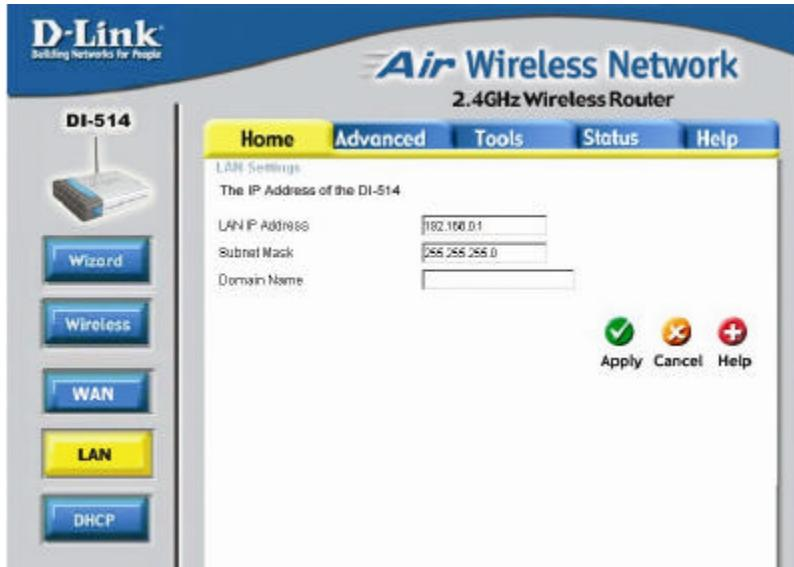
LAN is short for Local Area Network. This is considered your internal network. These are the IP settings of the LAN interface for the DI-514. These settings may be referred to as Private settings. You may change the LAN IP address if needed. The LAN IP address is private to your internal network and cannot be seen on the Internet.
